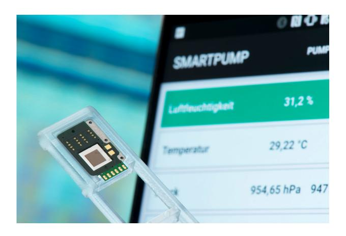
The world's smallest micromembrane pump measures just 25 square millimeters. Credit: Fraunhofer EMFT
