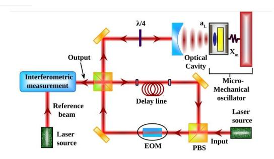
Proposed experimental setup to probe the effects of noncommutative structure. Credit: S. Dey et al. ©2017 Nuclear Physics B
