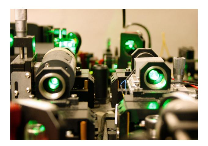
Partial view of the source producing the single photons that were stored in the quantum memory to produce entanglement between many atoms inside the memory. Credit: UNIGE
