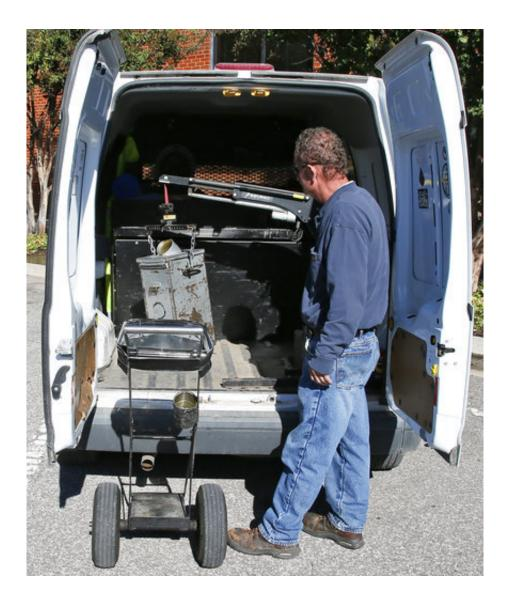
In this Wednesday, Oct. 11, 2017 photo, Wade Beal, parking meter technician, uses a small crane in the back of his vehicle to remove the can which holds coins from parking meters, in Oklahoma City. When full of coins the can can weigh 212 pounds. Oklahoma City, where the parking meter was invented 92 years ago, is doing away with the last few hundred of its coin-operated machines.(AP Photo/Sue Ogrocki)
