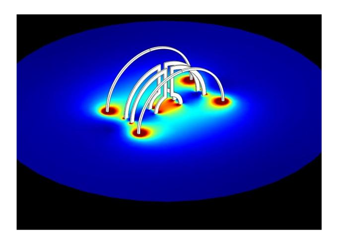
Two Lenz lenses are arranged in a Helmholtz coil pair. Simulation shows how the Lenz lenses focus magnetic flux. Credit: Nils Spengler/KIT
