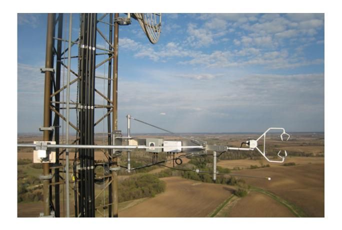
This image showcases the tower and instrumentation used to collect nitrous oxide emission data. Credit: University of Minnesota
