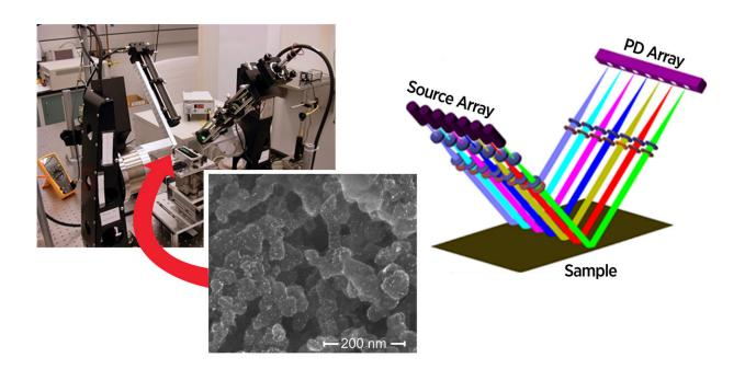
Well-controlled illumination allows the team's prototype device (top left) to scan thin layers of liquid containing platinum nanoparticles (lower center), a catalyst used in fuel cells. Scaling up the approach (right) could help meet industry's quality-control needs. Credit: M. Stocker / NIST
