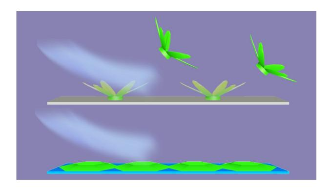
Renderings of ice crystals growing upward from a water-repellent surface (top) and along a water-absorbent surface (bottom). Credit: *Proceedings of the National Academy of Sciences*
