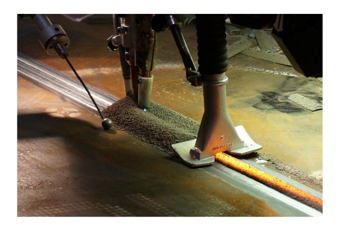
As shown, the submerged arc welding features a significantly wide groove with high inherent residual stresses. Credit: DTU/Daniel Sommerlund Pedersen
