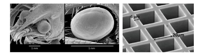
The Goddard-provided soft X-ray Wide-Field Imager proposed for a mission called ISS-TAO borrows heavily from nature. The images on the left and center show close-up views of a crustacean's eyes; the image on the right shows a manmade microchannel plate. Both operate the same way. Both gather light from multiple angles, focusing it into a single image to provide a wide field of view. Credit: J. Camp
