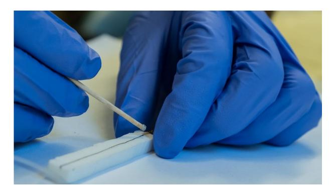
Rice University graduate student Amram Bengio prepares a sample nanotube fiber antenna for evaluation. The fibers had to be isolated in Styrofoam mounts to assure accurate comparisons with each other and with copper. The Rice fibers made only of carbon nanotubes may be practical antennas for aerospace applications and wearable electronics. Credit: Jeff Fitlow/Rice University
