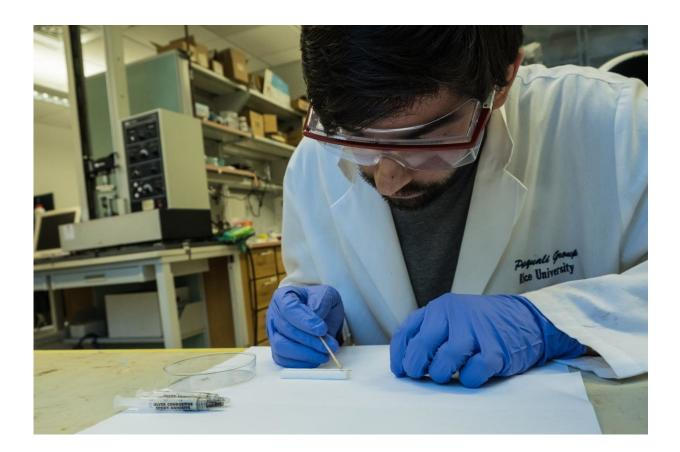
Rice University graduate student Amram Bengio sets up a nanotube fiber antenna for testing. Scientists at Rice and the National Institute of Standards and Technology have determined that nanotube fibers made at Rice can be as good as copper antennas but 20 times lighter. Credit: Jeff Fitlow/Rice University
