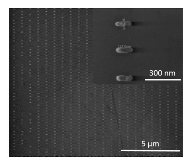
SEM images of nanoantenna array and in the inset a magnified view of the array elements. Credit: University of Bristol
