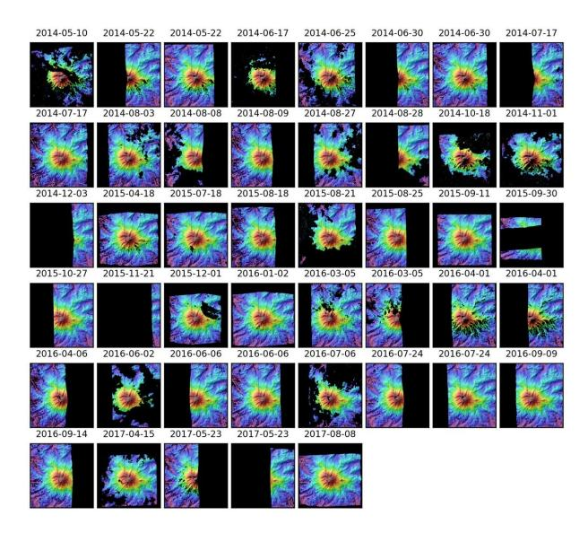
The full series of satellite elevation data for Mount Rainier from spring 2014 through summer 2017. The satellite-based instrument may or may not scan the entire mountain, and clouds can block portions of its view. Credit: David Shean/University of Washington
