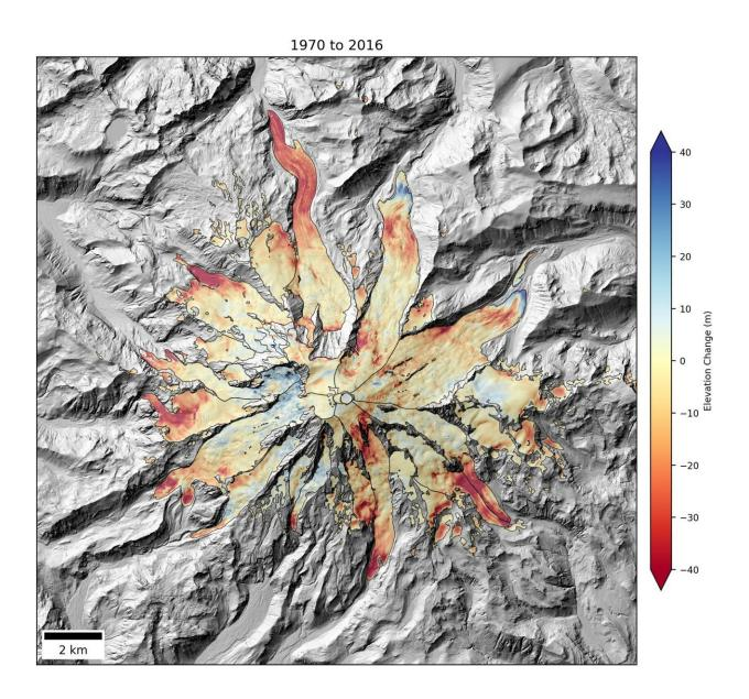
This map shows the elevation change of Mount Rainier glaciers between 1970 and 2016. The earlier observations are from USGS maps, while the recent data use the satellite stereo imaging technique. Glacier surface elevations have
