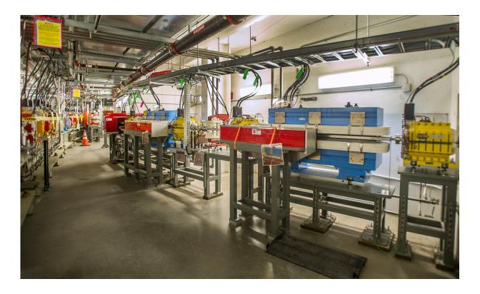
A view of the NSLS-II magnet girders, which help align the orbit of the electron beam. Credit: Brookhaven National Laboratory
