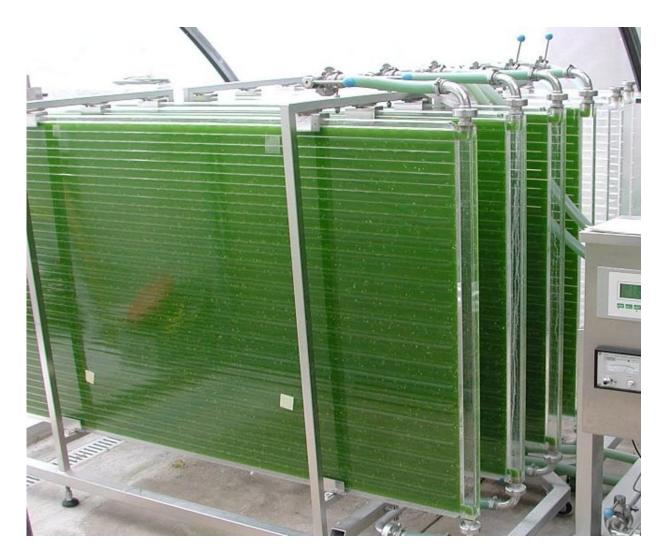
Photobioreactors produce algae using a light source and carbon dioxide. Credit: IGV Biotech, CC BY-SA
