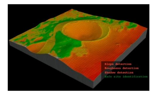
A map of a moon crater. A 'lidar' – the laser equivalent of radar – will be an essential part of ESA's autonomous landing and navigation system for Luna-27. Leia (Lidar for Extra-terrestrial Imaging Applications) will scan the surface of the moon with a laser for hazards such as slopes, boulders, craters and shadows. If the site seems too dangerous, the lander can decide to target a safer zone. Credit: European Space Agency
