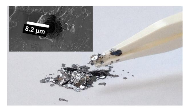
Kish graphite is a waste product from steel production. It could be used to make a cheap rechargeable battery out of abundant materials. Credit: Empa / ETH Zürich
