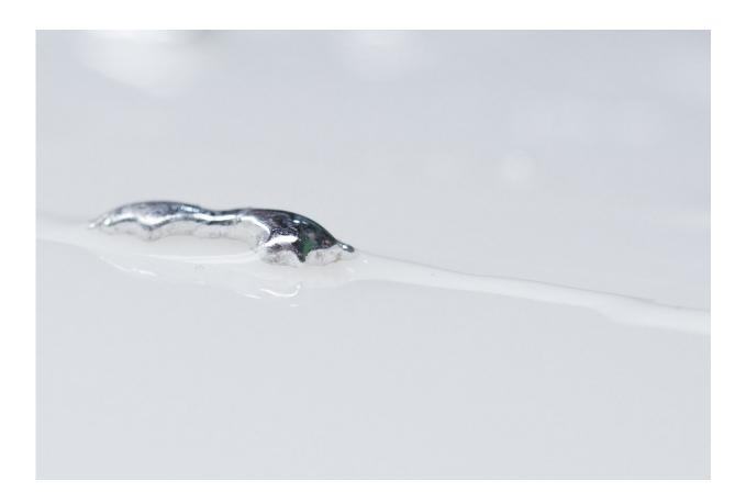
This image of a liquid metal 'slug' and its clear atom-thick 'trail' shows the breakthrough in action. When dissolved in a liquid metal core, certain metals leave behind this clear layer of their oxide, which is no thicker than a few atoms and can be peeled away by touching or rolling. Credit: RMIT University
