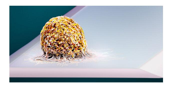
A human cell is attached to a cantilever: ETH Zurich researchers have developed a highly sensitive scale that measures the weight of a single cell. Credit: Martin Oeggerli, micronaut.ch / ETH Zurich / University of Basel
