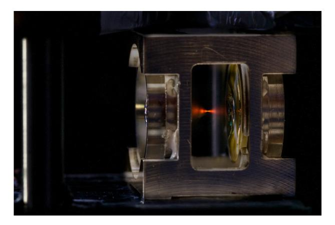
An imaging technique called 4Pi microscopy boosts resolution by sandwiching the sample between two strongly-focusing lenses. Quantum researchers have shown that borrowing this lens trick can boost interactions between photons and a single atom. Credit: Ale Cere / Centre for Quantum Technologies, National University of Singapore
