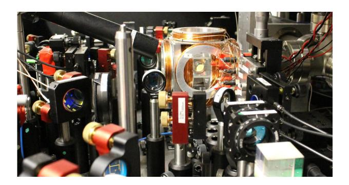
In the copper-encircled chamber at the centre of this setup at the Centre for Quantum Technologies in Singapore, photons bounce off a single atom. Controlling such interactions is important for quantum computing and metrology. Credit: Centre for Quantum Technologies, National University of Singapore
