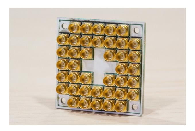
Intel's 17-qubit superconducting test chip for quantum computing has unique features for improved connectivity and better electrical and thermo-mechanical performance. Credit: Intel Corporation
