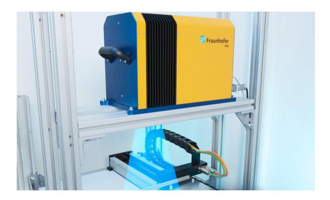
The fluorescence scanner – an imaging, inline measuring system – inspects components for impurities during the manufacturing process and identifies the exact point of contamination. Credit: © Photo Fraunhofer IPM
