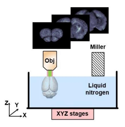
The cryo-MOST imaging system allows whole-brain mapping of senile plaques in the mouse brain. The system cools the sample by keeping it immersed in liquid nitrogen to enhance fluorescence from senile plaques. For whole-brain imaging, the XYZ stages move the sample to automatically alternate between imaging and the miller machine that removes a layer of the tissue each time the surface is imaged. Credit: Jing Yuan, Huazhong University of Science and Technology
