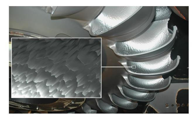
LMH Pelton turbine eroded by silt after one sediment season. Credit: Ecole Polytechnique Federale de Lausanne
