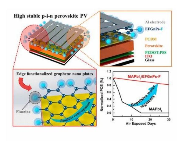
Highly stable p-i-n perovskite PV, prepared via a mechanochemical ball-milling method. Credit: UNIST
