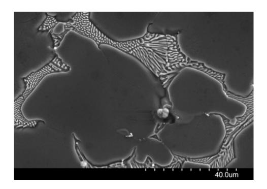
Image from electron microscope showing a large precipitate in magnesium alloy. These precipitates are dissolved through heat treatment, which substantially reduces the corrosion rate and makes the alloy very stable in the body. Credit: NYU Tandon School of Engineering
