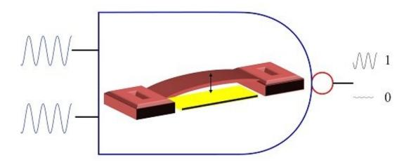
The cascadable, vibration-driven microelectromechanical logic gate takes electrical signals as inputs and produces a logic output (1 or 0) based on the resonance of the microbeam. Credit: © 2016 KAUST
