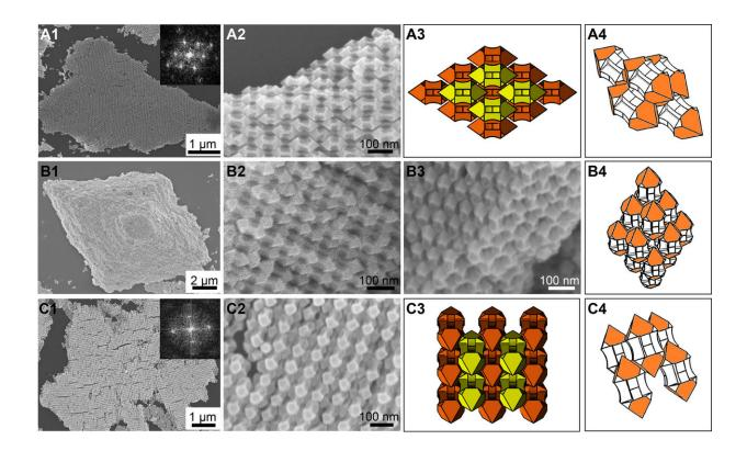
3D SCs assembled by GNAs. SEM images (A1, A2, B1, B2, B3, C1, and C2) and geometric models (A3, A4, B4, C3, and C4) of Net III (A1 to B4) and Weave III (C1 to C4) SCs. Insets show the corresponding FFT patterns. Facets lying against the facets of neighboring GNAs are painted in saffron in (A4), (B4), and (C4). Credit: Wang et al., *Sci. Adv.* 2017;3: e1701183
