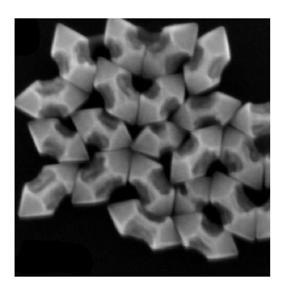
Scanning electron microscope image of gold nanoarrows. Credit: Wang et al., *Sci. Adv.* 2017;3: e1701183
