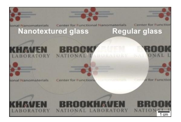
Glass surfaces with etched nanotextures reflect so little light that they become essentially invisible. This effect is seen in the above image, which compares the glare from a conventional piece of glass (right) to that from nanotextured glass (left), which shows no glare at all. Credit: Brookhaven National Laboratory
