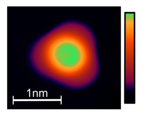
The top view shows: just one atom wide - less than a nanometre - is the wire (green), which is mounted vertically on a conductive platform (red). It can be easily attached to a metal surface (dark) like a suction cup - an electrical contact is realized. Credit: Jasper-Tönnies
