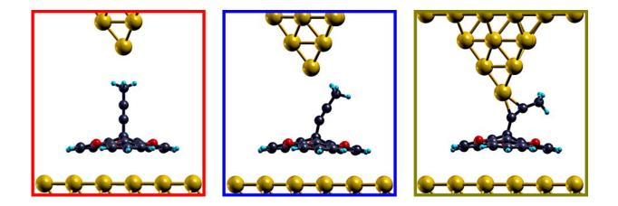
This is how the wire molecule becomes a nano switch: the closer the tip of the scanning tunnelling microscope (yellow) gets to the nano wire (blue), the more the wire bends - and the current flow changes. This is due to quantum mechanical forces acting between the tip and the wire. They change the geometry of the molecule, and thereby its properties. Credit: Jasper-Tönnies
