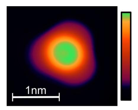
The top view shows: just one atom wide - less than a nanometre - is the wire (green), which is mounted vertically on a conductive platform (red). It can be easily attached to a metal surface (dark) like a suction cup - an electrical contact is realized. Credit: Jasper-Tönnies
