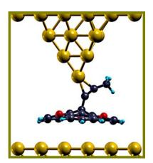
This is how the wire molecule becomes a nano switch: the closer the tip of the scanning tunnelling microscope (yellow) gets to the nano wire (blue), the more the wire bends - and the current flow changes. This is due to quantum mechanical forces acting between the tip and the wire. They change the geometry of the molecule, and thereby its properties. Credit: Jasper-Tönnies
