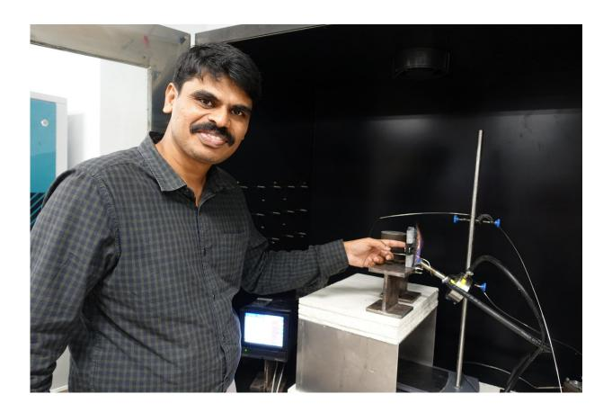
NTU Assistant Professor Aravind Dasari putting his finger on a piece of plastic that is cool enough to touch, which was placed behind a steel plate coated with FiroShield and exposed to a flame over 900 degrees Celsius. Credit: Nanyang Technological University
