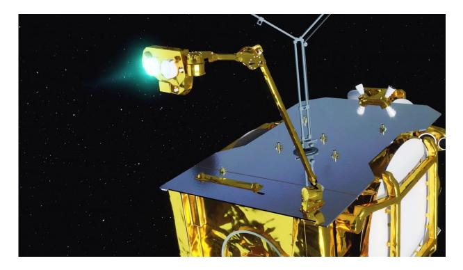
Eutelsat-172B is equipped with a pair of 3 m-long three-jointed arms carrying electric propulsion thrusters at the end. Instead of thrusters embedded at the corners of the satellite, these twin arms can be moved freely about its body so their thrusts can always be aligned precisely with the satellite's centre of gravity for orbit raising and stationkeeping – saving propellant to elongate mission life. Credit: Airbus Defence and Space
