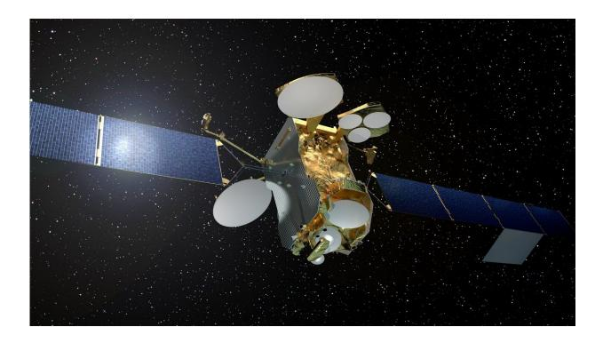
Eutelsat-172B is the first European telecommunications satellite to demonstrate electric propulsion for orbit-raising and stationkeeping in geostationary orbit. The satellite is equipped with two articulated thruster arms. Credit: Airbus Defence and Space
