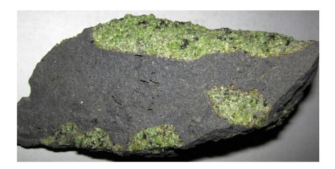
Olivine is the primary component of Earth's upper mantle, which comprises the bulk of the planet's tectonic plates. A new study gives researchers a better idea of olivine's strength, with implications for how tectonic plates form and move. Credit: John St. James/Flickr
