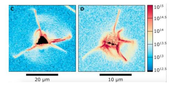
These examples of nanoindentation experiments using pyramidal (left) and spherical (right) indenter tips show how the mineral olivine deforms in response to a given load. Credit: University of Pennsylvania
