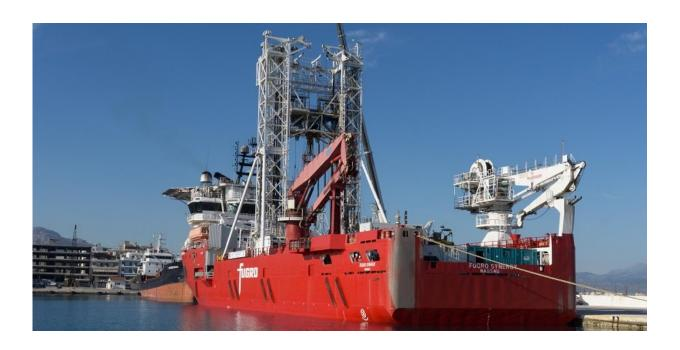
Drilling Vessell Fugro Synergy will extract samples from 750 metres below the
