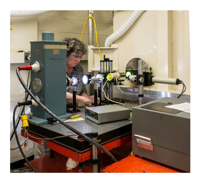
NIST physicist Gillian Nave adjusts alignment of the light beam that passes from the xenon source at left, through the absorption cell (center, wrapped in brown
