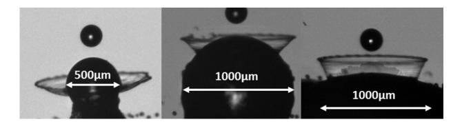
Examples of initiation of crown rim instability. By the time the instability has appeared on the crown rim, the original droplet has collapsed on the particle. Credit: Hardalupas and Charalampous
