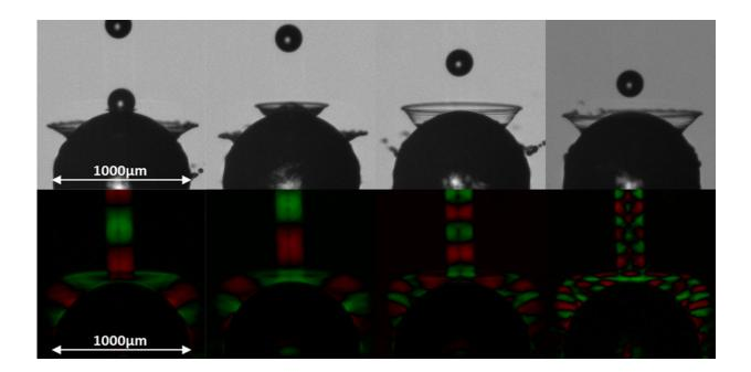
Example of the droplet impingement sequence. Top row: Example images from the dataset. Bottom row: Showing progressively finer details of the droplet-particle impingement process. Credit: Hardalupas and Charalampous
