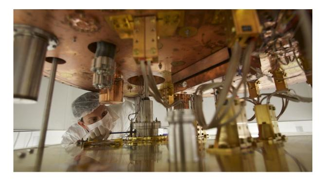
A researcher works on the cryostat unit for CUORE during the assembly process. Credit: CUORE collaboration
