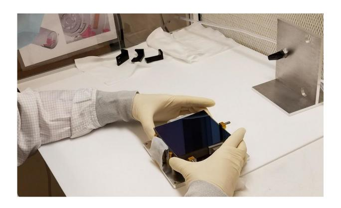
The DEUCE grating, sensitive to ultraviolet, is carefully positioned for bonding into its flight mount. Credit: Nicholas Erickson
