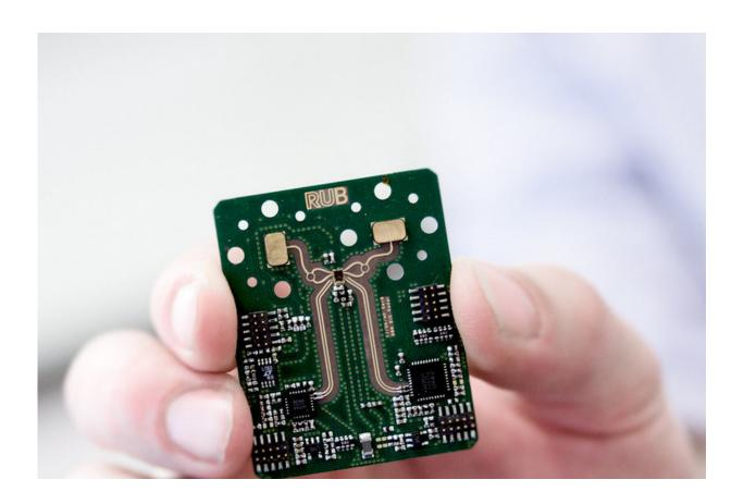
Developed by the Institute of Integrated Systems in Bochum, the radar sensor is no bigger than this. Credit: © Roberto Schirdewahn
