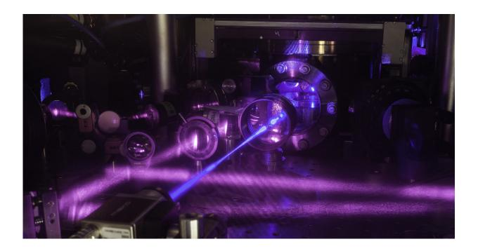
JILA's three-dimensional (3-D) quantum gas atomic clock consists of a grid of light formed by three pairs of laser beams. Multiple lasers of various colors are used to cool the atoms, trap them in a grid of light, and probe them for clock operation. A blue laser beam excites a cube-shaped cloud of strontium atoms. Strontium atoms fluorescence strongly when excited with blue light, as seen in the upper right corner behind the vacuum window. Credit: G.E. Marti/JILA
