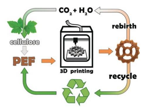
In our modern world, eliminating plastics is inconceivable. Unfortunately, they do have disadvantages, including the formation of CO2 in both production and combustion, depletion of fossil feedstocks, and growth of landfills. In the journal *Angewandte Chemie*, Russian researchers introduce a new way forward, a polymer made entirely from biomass that can easily and inexpensively be used in 3-D printing. Objects produced in this way are of high quality, easily recyclable, and
