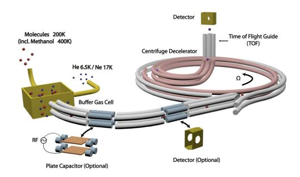
Schematic view of the experimental setup of the "cryofuge". Credit: MPQ, Quantum Dynamics Division
