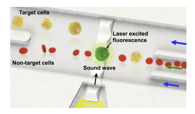
Schematic of the fluorescence activated sorting of a single target cell in a heterogenous cell sample. Credit: SUTD/Ye Ai
