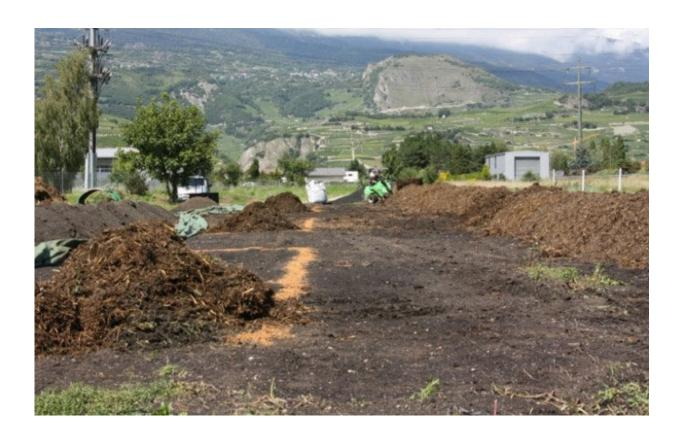
Field experiment in Switzerland, with setup of compost windrows from mixed manure before adding the biochar. Credit: Nikolas Hagemann/University of Tübingen
