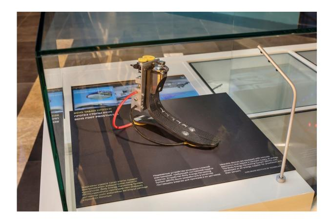
Systems converting energy of the body into electricity, such as this foot prosthesis, are to be used by KIT scientists to power portable electric devices, such as smartphones or pacemakers of the heart. Credit: KIT/Andreas Keller, courtesy KUNZBERG GmbH
