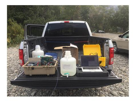
MBARI's third-generation Environmental Sample Processor is small enough to fit in a fishing tackle box. The entire monitoring setup is shown here in the back of a pickup truck near one of the team's field sites in Montana. Credit: Kevan Yamahara © 2017 MBARI
