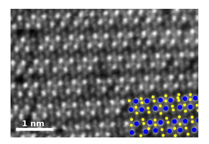
A high-angle annular dark-field image of pure rhenium diselenide. In the key at bottom right, rhenium atoms are blue and selenium atoms yellow. Credit: Oak Ridge National Laboratory
