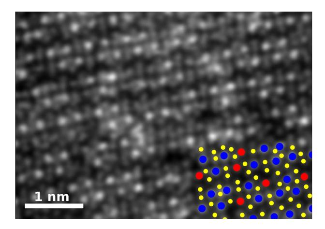
An image of rhenium-doped molybdenum diselenide shows how the material's atomic structure has been rearranged by the addition. The key shows the positions of rhenium atoms in blue, selenium in yellow and molybdenum in red. Credit: Oak Ridge National Laboratory
