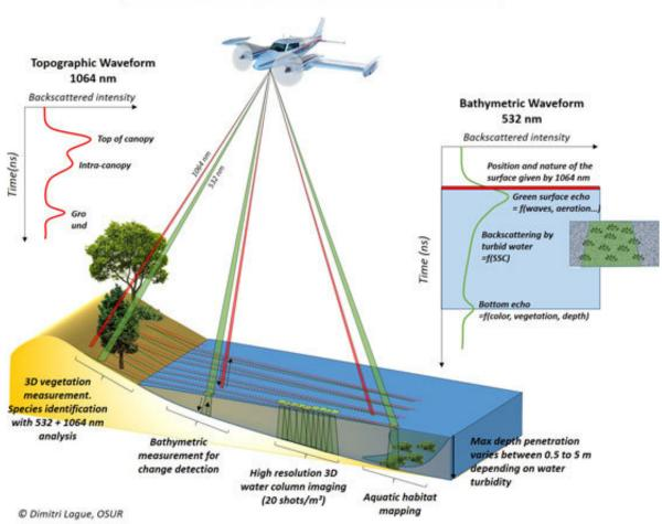
Full Waveform topo-bathymetric Airborne Lidar
