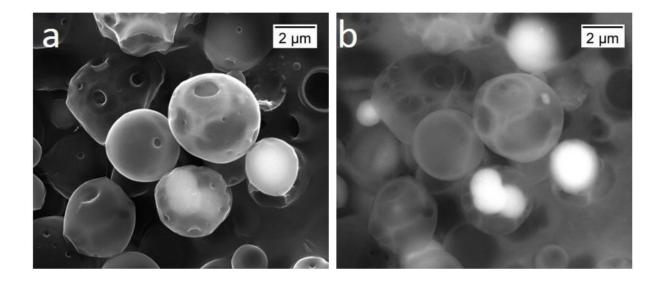
SEM images (obtained from the BSE detector) of PLA-coated micro-particles with various mass ratios of CaCO3 particles relative to PLA (a) 0, (b) 0.2. Credit: Tomsk Polytechnic University (TPU)
