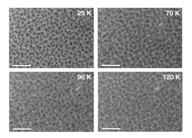
UV-irradiated amorphous water ice observed by a transmission electron microscope as the temperature rose (25K/-248C/-414F, 70K/-203C/-333F, 96K/-177C/-287F, 120K/-153C/-243F). Amorphous water ice islands (the dark areas in the photos) change shape and spread over the substrate like liquid, which is indicated by the blurring of the images. Scale bars=0.5 micrometers. (Tachibana S., et al., Science Advances, September 30, 2017) Credit: Tachibana S., et al., *Science Advances*, September 30, 2017
